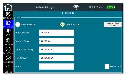
Figure 10 - IP specifications (Static IP)
