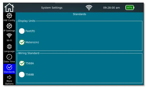
Figure 17 - Setting the units and cabling standards
