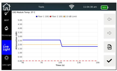
Figure 61 – LiveLight measurement finished
