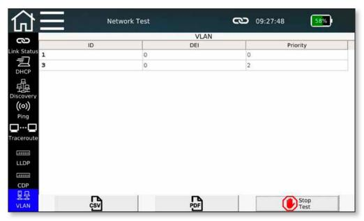
Figure 50 - VLAN detection
