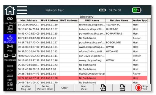
Figure 46 - Network detection (list display with duplicate IP address)
