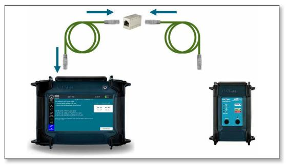
Figure 39 - Test setup for setting the reference - Cu
