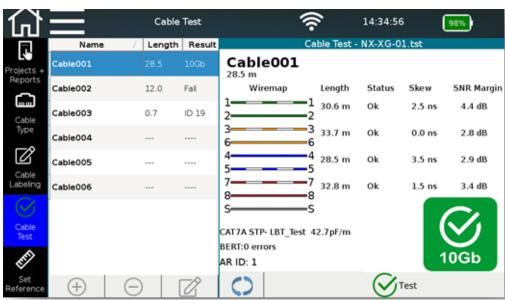
Figure 25 - Cable test screen after successful test run - Cu
