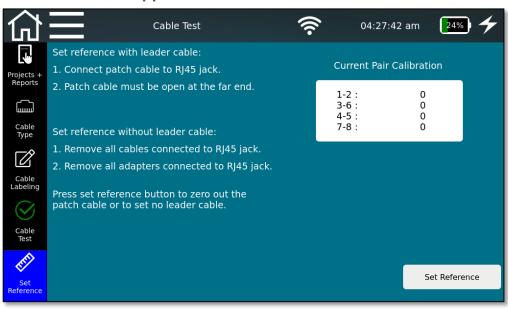
Figure 38 - Setting reference with or without test cords - Cu
