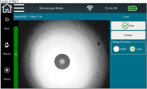
Figure 35 — Microscope test of a connector end face
