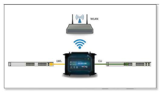
Figure 42 - Test setup for connecting to an active network
