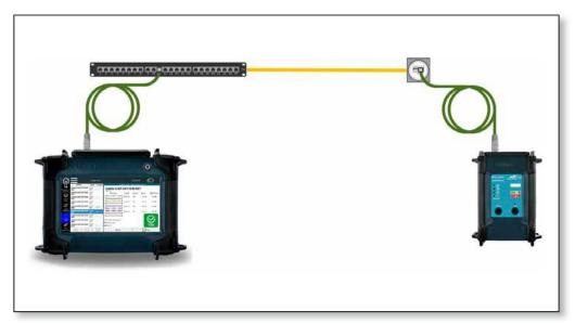
Figure 32 - Test setup for passive qualification test on copper links
