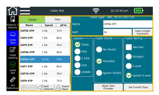
Figure 28 - Cable types and test parameters - Cu
