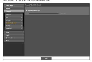
Select **Network Bandwidth limit** and then specify the maximum bandwidth. The camera will not be able to use more than the specified limit in the event of network traffic.
