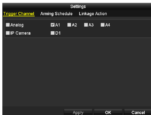
Figure 8.15 Set Triggering Channel of VCA Alarm
